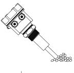
When material touches the rod, vibration stops as resonance gets disturbed.
